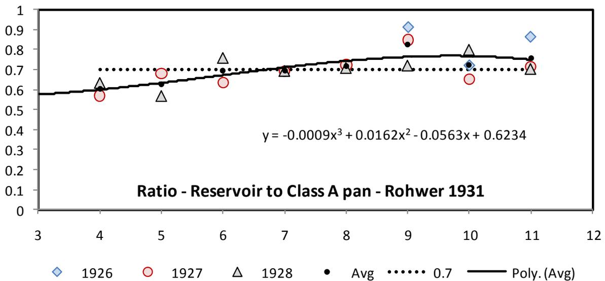
Fig. 6. Ratios of evaporation from a 85-ft (27.9 m) diameter reservoir in Fort Collins to Class A pan evaporation located adjacent to the reservoir (Rohwer 1931).
